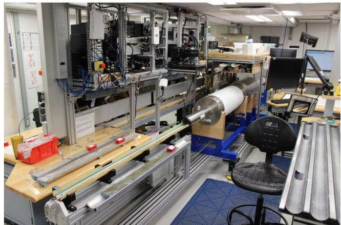
Paleomagnetism lab on the JOIDES Resolution. Cryogenic rock magnetometer in center of image
